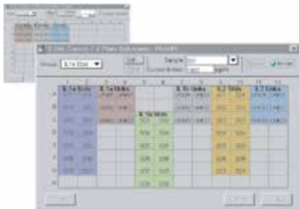
Figure 1. Flexible template assignment. Standards for multiple calibration curves and unknowns can be run on separate plates.
