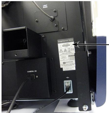
Figure 1-1: Serial Number location on the back of your ImageXpress instrument
