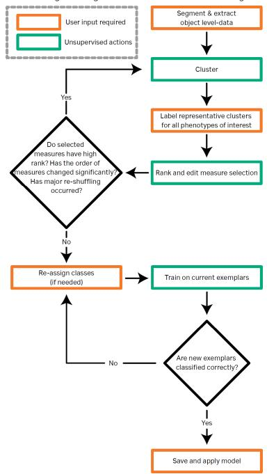
The following flow diagram shows the workflow when using IN Carta Phenoglyphs.
