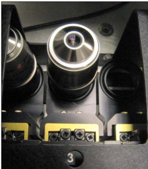
9. Replace the objective with the correction collar correctly set (if applicable).
