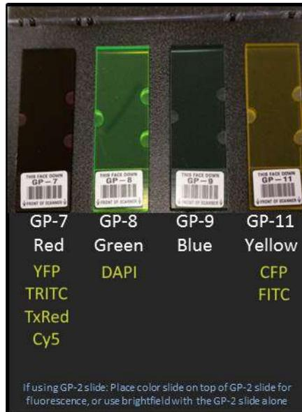
GP slide compatibility for IX Confocal HT.ai
