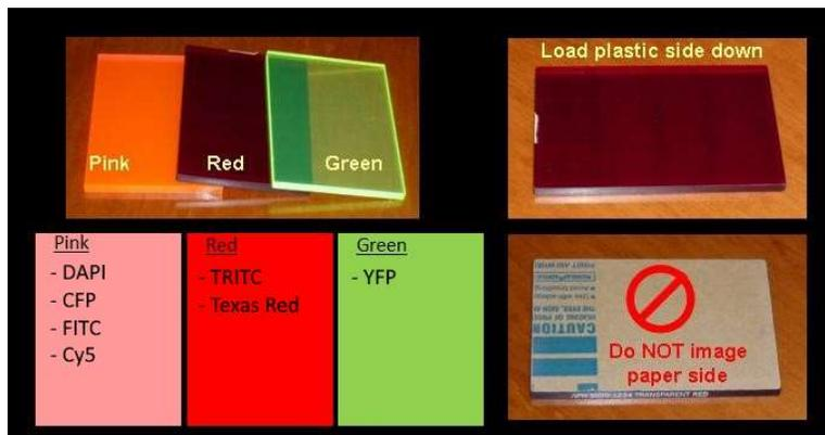
Shading plate compatibility for IX Confocal HT.ai
