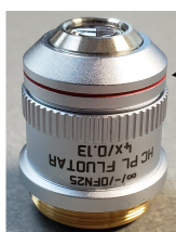
Color Band on 4x Objective
