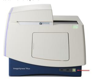
When the status light on the power button is off, the instrument is fully powered off.
