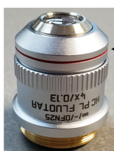
Color Band on 4x Objective
