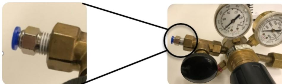
If your regulator terminates with a ¼" NPT male fitting, you will need to provide a ¼" NPT female to ¼" NPT female connector, as shown below.
