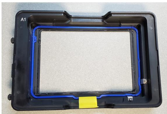
The plate skirt height adapter sits inside the environmental control cassette to raise the plate, which can help autofocus succeed. When you use the adapter, you must select a labware specification that adds 1.5 mm to the actual **Plate Height** value. See the *CellReporterXpress Help* or the *CellReporterXpress User Guide* for details on adding and selecting a labware specification.
