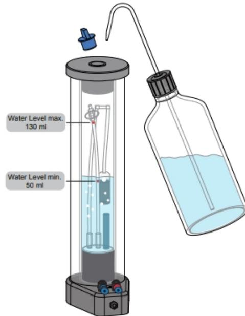
The humidifying column holds 130 ml (4.4 oz) of ultrapure water, which is enough to continuously provide humidity for up to 72 hours. When the water level approaches the minimum indicator (approximately one-third full), add 18 Mohm•cm ultrapure water to reach the maximum level.
