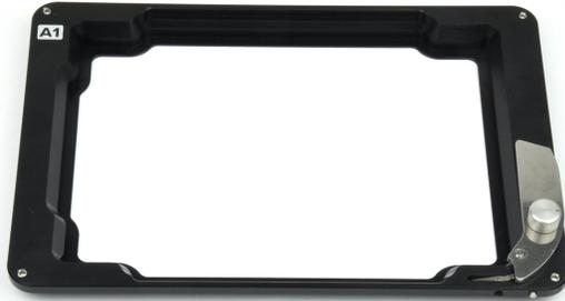
The plate holder is designed for imaging multi-well microplates in standard ANSI (SBS) formats with plastic or glass bottoms and standard footprint dimensions. It can also be used with the optional dish holder, which holds up to six 35 mm (1.38 in.) dishes. Optimal image quality depends on plate flatness, well bottom thickness, and optical clarity.
