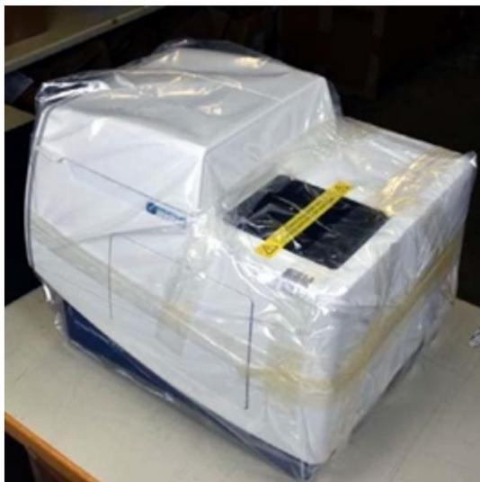
11. With one person on each end, place the instrument in the bottom foam packing as shown below.
