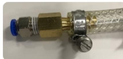
It is also possible that your lab gas line terminates with a line regulator. In this case, attach the 1/4" NPT male to 6 mm O.D. Push-to-Connect fitting directly to the line regulator.
