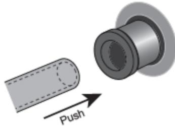
3. After inserting the tubing, gently pull the tubing to confirm it is seated.
