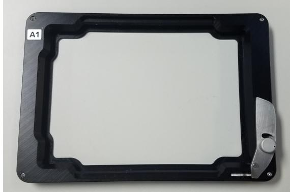
The plate holder is designed for scanning multi-well microplates in standard ANSI (SBS) formats with plastic or glass bottoms. It can accommodate other plate formats that have standard microplate footprint dimensions. For example, glass slides can be imaged using a slide adapter included in the accessory kit. Optimal image quality depends on plate flatness, well bottom thickness, and optical clarity.
