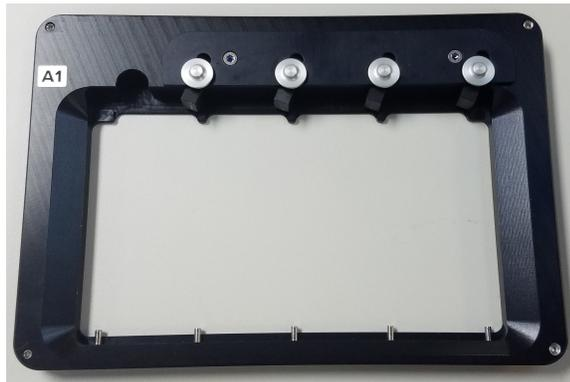
The slide holder holds four standard microscope slides of 25 mm x 75 mm (1 in. x 3 in.).
