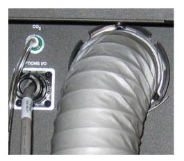
Figure 7-3: Environment Control option warm air hose and carbon dioxide tubing on the back of the ImageXpress Nano System
