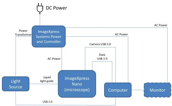
Figure 3-1: ImageXpress Nano System Components Without Options Using MetaXpress<sup>®</sup> Software
