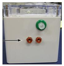
Figure 7-8: Water level sensor wire sockets
