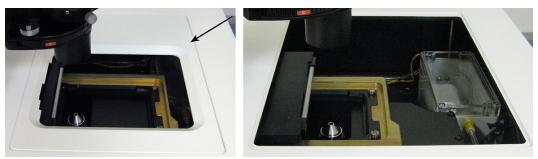
Figure 7-10: Access panel around the top door on and off
