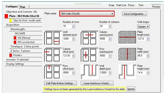
Figure 5-8: Plate Acquisition Setup Dialog with Warning Icons
