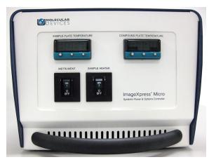
Figure 7-1: ImageXpress Systems Power and Options Controller used for the ImageXpress Nano System
