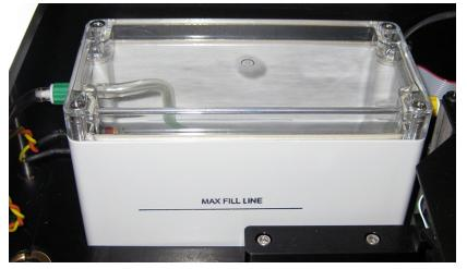
Figure 7-11: ImageXpress Environmental Control option water reservoir
