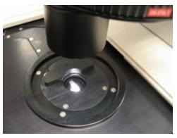
Figure 7-16: Transmitted Light shutter
