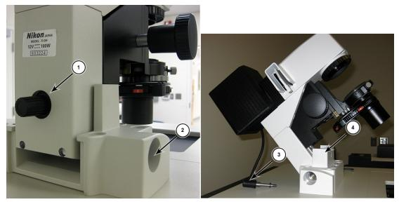
Figure 7-17: Hinge-release knob and hinge
