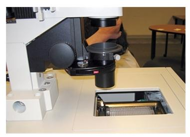
Figure 7-15: ImageXpress System with Transmitted Light option (detailed view)
