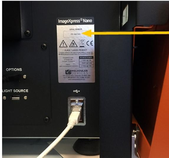
**Figure 6-3: Serial Number location on the back of the ImageXpress Nano System**
