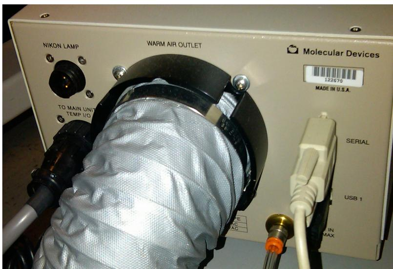
**Figure 1-3:** Environment Control option warm air hose and carbon dioxide tubing on the back of the Environmental Control Option Controller
