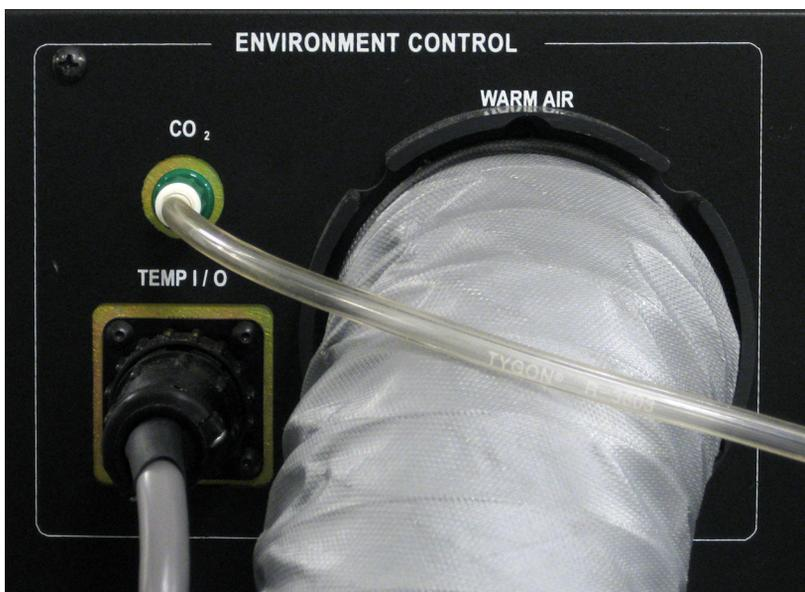
**Figure 1-4:** Environment Control option warm air hose and carbon dioxide tubing on the back of the ImageXpress Micro Standard System
