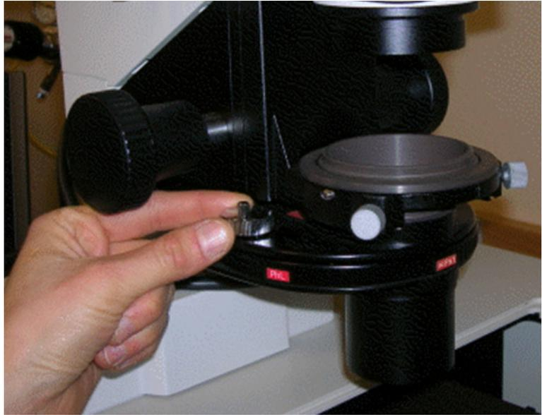
**Figure 4-22:** Centering the condenser annulus ring with the objective phase ring
