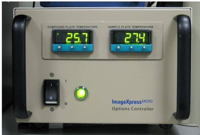
**Figure 1-1:** Environmental Control Option Controller used for the ImageXpress Micro Standard and XLS Systems
