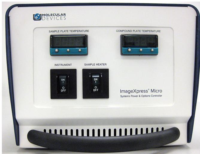
**Figure 1-2:** Systems Power & Options Controller used for the ImageXpress Micro Confocal System
