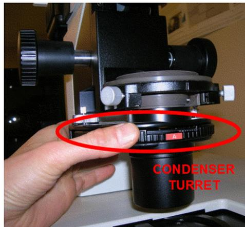
**Figure 4-15:** Condenser turret with position A at the front
