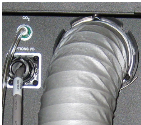
Figure 7-3: Warm Air Hose and CO 2 Tube on the Back of the ImageXpress Micro Confocal System
