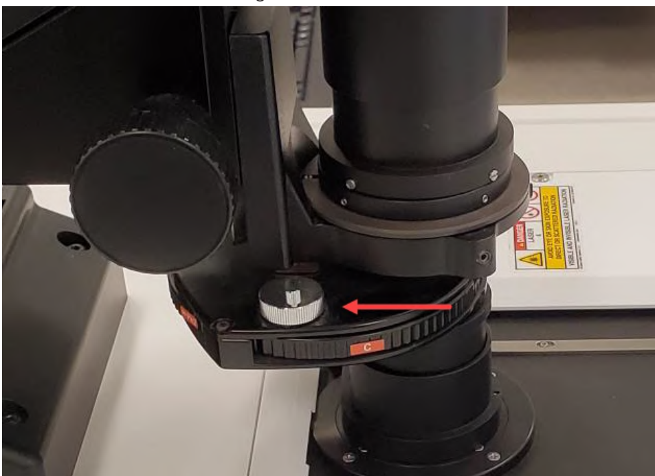
Figure 7-64: Centering the Condenser Annulus Ring with the Objective Phase Ring
