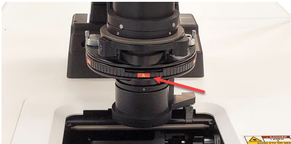
Figure 7-57: Condenser Turret with Position A at the Front
