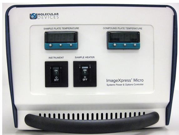
Figure 7-1: ImageXpress Systems Power and Options Controller for the ImageXpress Micro Confocal System
