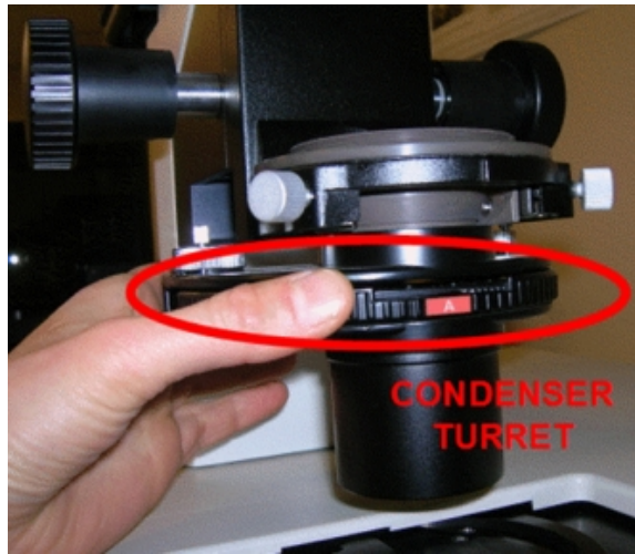
Figure 7-54: Condenser Turret with Position A at the Front
