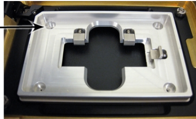
Figure 3-16: Loaded Metal Slide Holder Plate with Integrated A1 Well Pinhole
