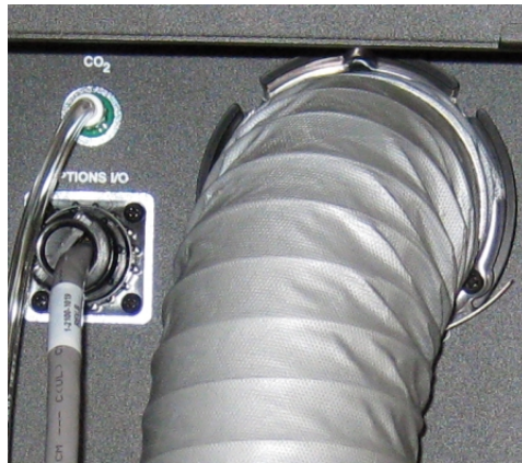
Figure 7-3: Environment Control Warm Air Hose and Carbon Dioxide Tube on the Back of the ImageXpress Micro Confocal System
