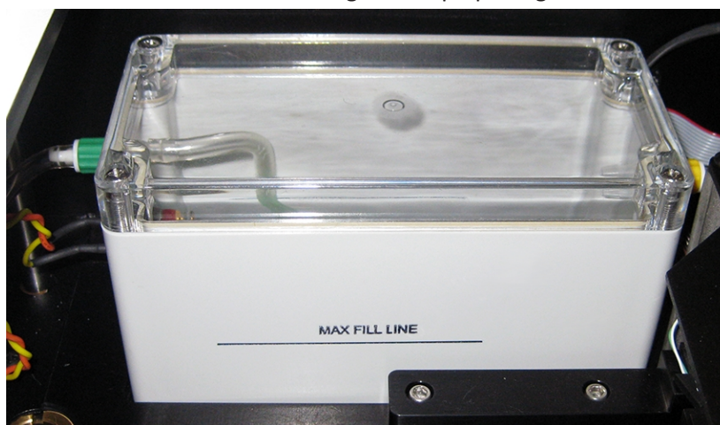
Figure 7-11: ImageXpress Environmental Control Option Water Reservoir
