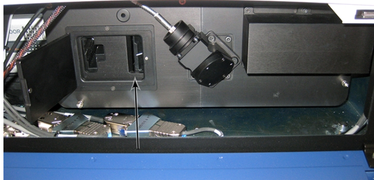
Figure 8-24: Confocal Module Housing with Filters Access Door Open
