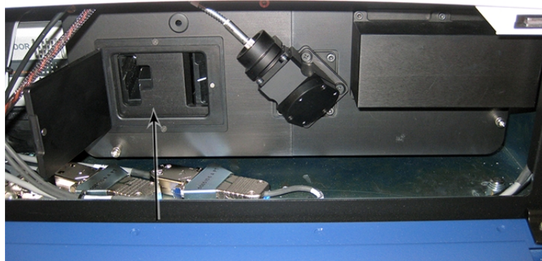
Figure 8-17: Confocal Module Housing with Filters Access Door Open
