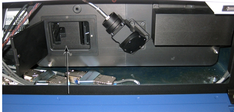
Figure 8-13: Confocal Module Housing with Filters Access Door Open
