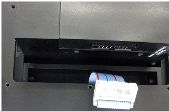
Figure 8-3: Ribbon Cable and Cable Socket on the Bottom of the Disk Box
