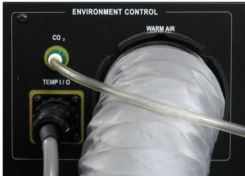
Figure 8-6: Environment Control option warm air hose and carbon dioxide tubing on the back of the ImageXpress Micro Standard System
