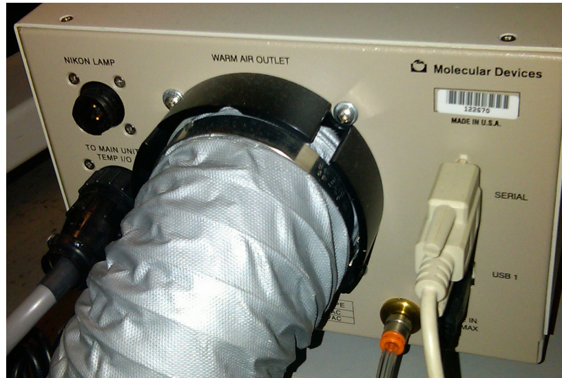
Figure 8-5: Environment Control option warm air hose and carbon dioxide tubing on the back of the Environmental Control Option Controller used for the ImageXpress Standard, XL, and XLS Systems
