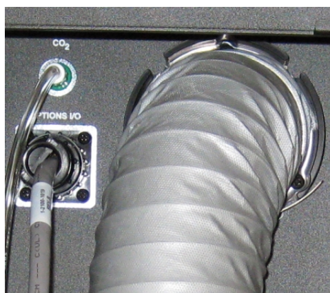
Figure 8-4: Environment Control option warm air hose and carbon dioxide tubing on the back of the ImageXpress Micro 4 System
