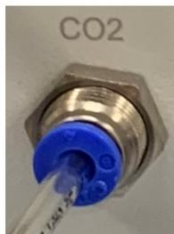
5. Remove the Gas Control Speed Valve from your CO<sub>2</sub> gas source.
