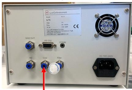
5. On the back of the gas mixer, connect a 1 inch piece of the provided 4 mm tubing to the **GAS OUT** port.
