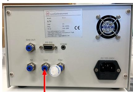
4. On the back of the gas mixer, connect a 1 inch piece of the provided 4 mm tubing to the **GAS OUT** port.
