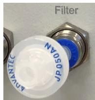
The **Filter** inlet port pumps in ambient air for O<sub>2</sub> use in your gas mix.
