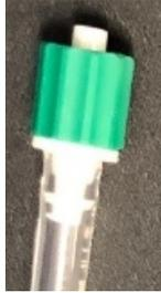
then connect the tubing over the 4 mm tubing connected to the **GAS OUT** port on the back of the gas mixer.
