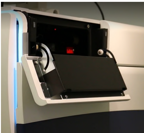
Figure 7-12: Right Side Upper Access Door
