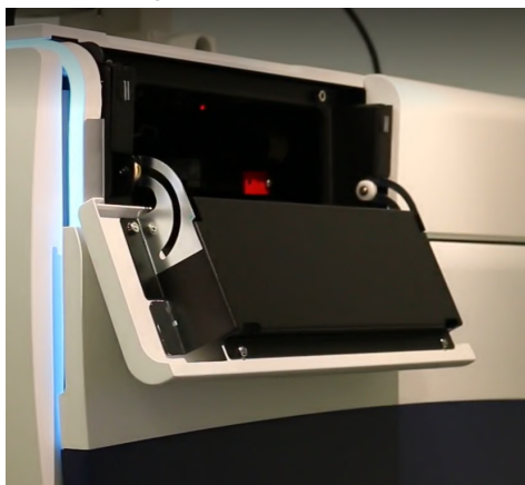
Figure 7-16: Right Side Upper Access Door
