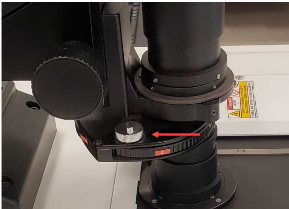
Figure 7-49: Centering the Condenser Annulus Ring with the Objective Phase Ring
