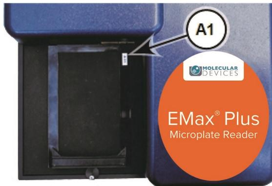
3. Select the **Home** tab and click
