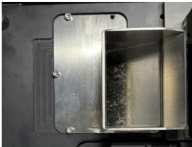
Looking inside the instrument, you can see the top of the slide to confirm that it is clear of obstructions.
