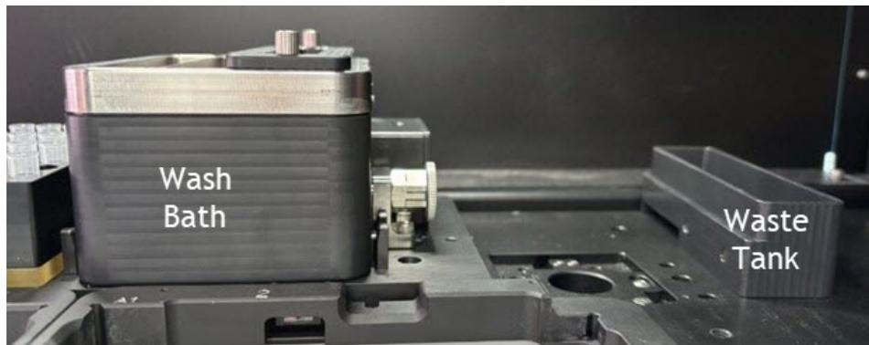
To reattach the liquid waste tank to the wash bath, hold the liquid waste tank to the right side of the wash bath and the magnet will guide the liquid waste tank to the proper position.
