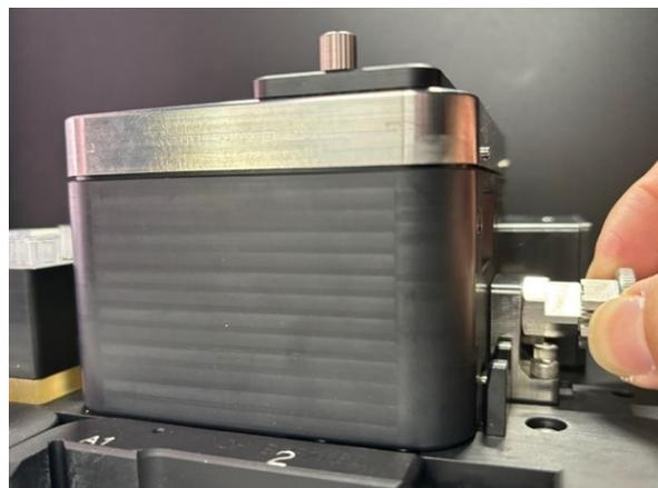
3. Lift the wash bath off of the instrument deck.
