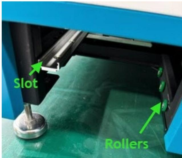
Align the drawer cover with the slot and roller rails inside the instrument.
