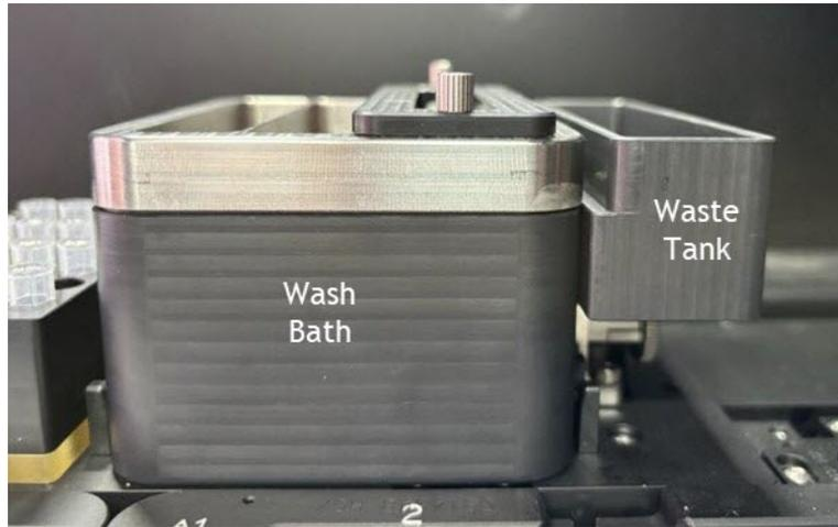
Pull the liquid waste tank to the right to remove it from the wash bath.
