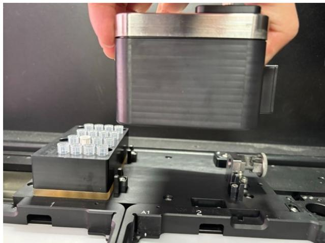
4. On top of the wash bath, unscrew the hand screws that keep the sponge holder in the wash bath.
