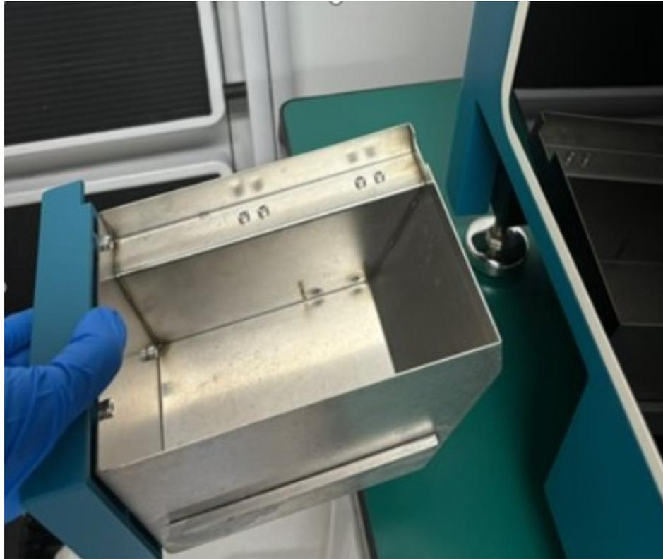
The drawer opening has a slot on the left and rollers on the right.
