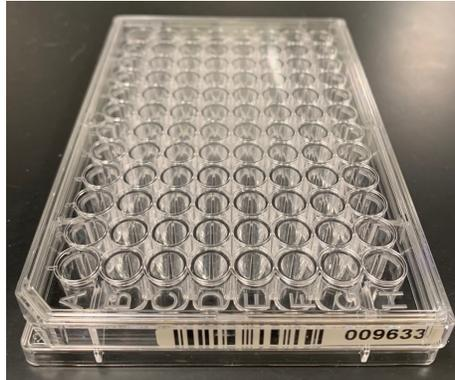
When you use a 2D code reader, use the 2D code type Data Matrix barcode (ISO/IEC 16022) which is a high-density, two-dimensional (2D) symbology that encodes text, numbers, files, and actual data bytes. (Tested for 5 mm and 7 mm codes.)
