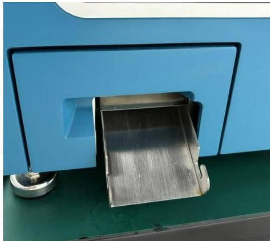
The end has notches to which to attach a waste bag.
