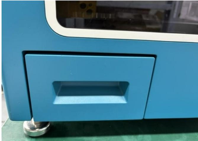
The drawer is a closed box that does not have a filled sensor. Look inside the instrument to see the tips and pins that have been discarded.
