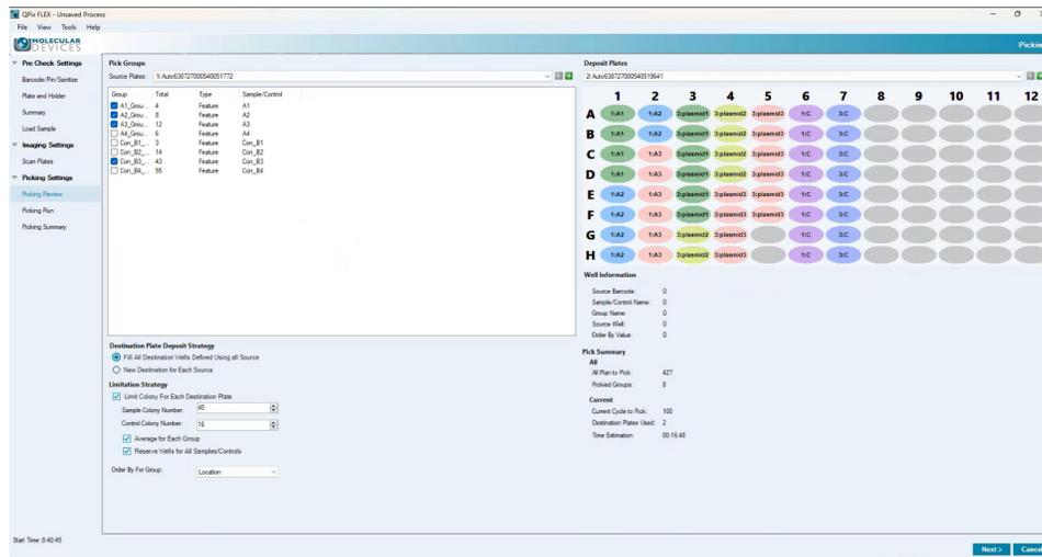
The left side displays the source plates, and the right side displays the destination plates.
