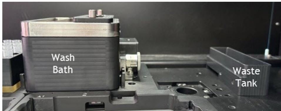
2. On the wash bath, pull the lock pin out to unlock the wash bath from the instrument deck.
