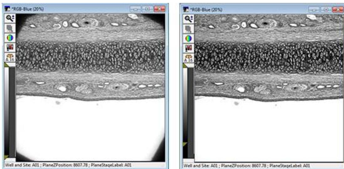
**Figure 8-58: Adjustment of the Field Aperture Diaphragm Comparison**
