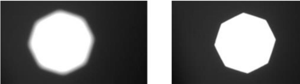
**Figure 8-57: Condenser height focus adjustment comparison**
