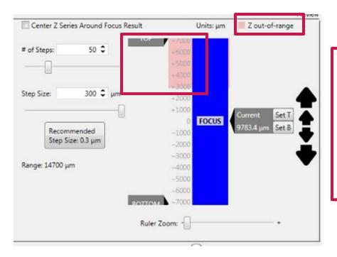
If Step Size and/or # of Steps results in the Z-series being outside of the physical range of the objective, a pink overlay will appear. Reduce the **# of steps**, adjust **Step Size** or set z-series to a position to below the pink area to get rid of the error
