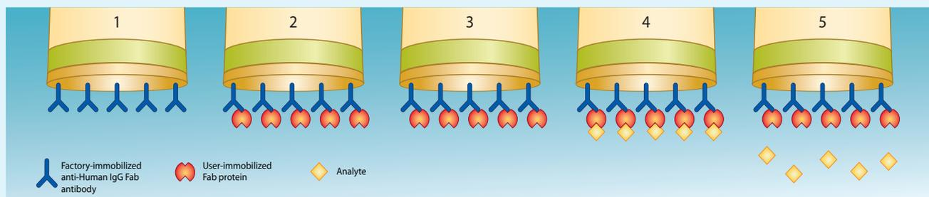
**FIGURE 1:** Example workflow for kinetic characterization of the interaction between a GST fusion protein and a target analyte. The assay consists of 5 assay steps. Step 1: equilibration, Step 2: loading (capture) of GST-fusion, Step 3: baseline, Step 4: association kinetics, Step 5: dissociation kinetics.
