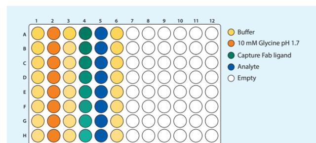
**FIGURE 2:** Example plate map for a kinetic assay that includes a pre-conditioning cycle, ligand loading, association, dissociation and a regeneration cycle. An assay step list using the sample plate is described in Table 1. The same sample wells (column 3) are used for the baseline and dissociation steps for optimal use of the inter-step correction processing feature.
