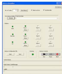
Figure 1 AutoRun Control Screen allows simple configuration of automated runs with result file destination, event logging and error notification. System status and control are also displayed.
