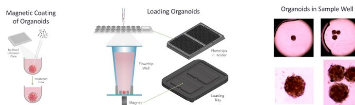
Figure 2. Schematic of the protocol for magnetic labeling and positioning of PDOs. Transmitted light images of PDOs are shown on the Right. PDOs are centered in the wells with no optical artifacts from NS particles.
