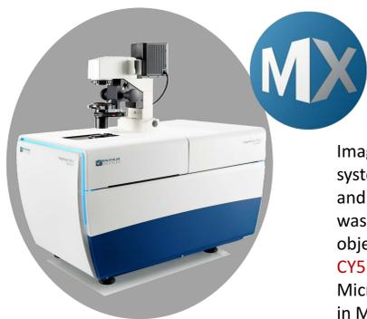
ImageXpress® Micro Confocal high content imaging system (Molecular Devices) equipped with widefield and spinning disk confocal optics (60 μm pinhole) was used to acquire images with 20X, 40X or 60X air objectives using filter cubes for DAPI, FITC, TRITC, & CY5 wavelengths. The images were analyzed with a Micronuclei Application Module or a Custom Module in MetaXpress® software.
