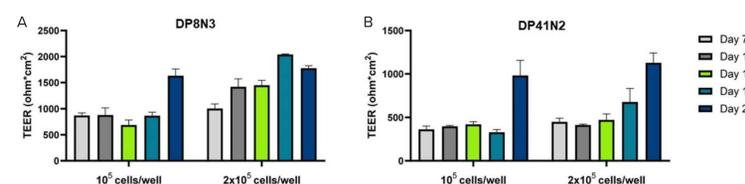
Figure 3. TEER values of monolayers derived from (A) DP8N3 or (B) DP41N2 organoids were measured 7, 10, 14, 17 and 21 days after seeding. Values were determined taking into account blank resistance from inserts with no cells and the culture insert area. Data are expressed as means ± SD (n=3).
