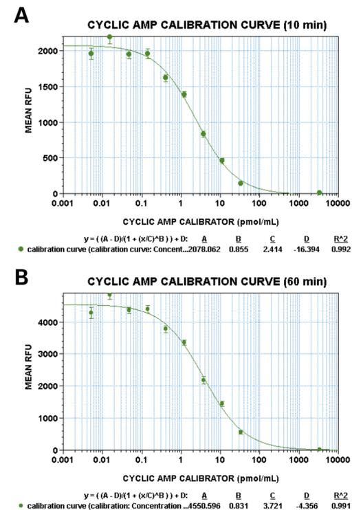
Figure 1. Dose response curves for cAMP calibrator using Gemini XS. Dose responses are shown for (A) 10 minutes and (B) 60 minutes after addition of Stoplight Red substrate. Each point on the dose response curves represents the average of eight replicate samples. The error bars denote the standard deviation from the mean. The R<sup>2</sup> value is 0.99 for a 4-parameter curve fit. RFU denotes relative fluorescence units.
