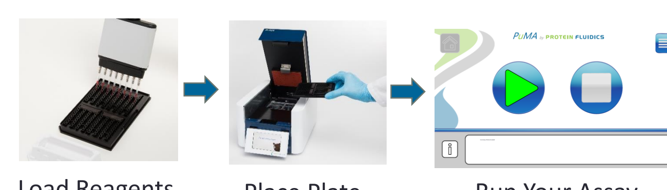
Figure 4. ELISA workflow for automated Pu-MA System and cartoon of automated assay steps in an ELISA protocol. The microfluidic assay channel provides solid support for the capture antibody.
