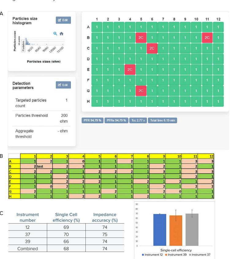
**Figure 6.** A. Impedance peak values generated by the DispenCell software for a 96-well plate after dispensing CHO-GFP cells and analysis B. CSI-FL Day 0 manual counts from images for the same plate using GFP detection for Day 0 count assurance. C. Averages of single-cell efficiency and Impedance accuracies of 96-well plates of individual instruments and an average of the instruments and representation of Single-cell efficiency (%) of all three instruments based on Day 0 images.
