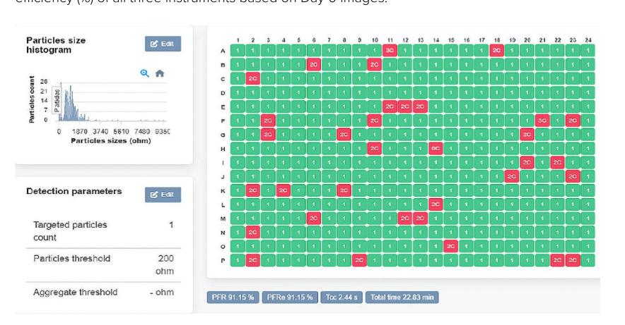
Figure 7. Impedance peak values generated by the DispenCell software for a 384-well plate after dispensing analysis
