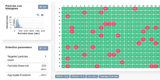
Figure 7. Impedance peak values generated by the DispenCell software for a 384-well plate after dispensing analysis
