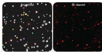
Figure 1. The ClonePix 2 System reveals diverse levels of fluorescent intensity with CHO-M1 cell line, demonstrating it can distinguish between various levels of expression of GPCR M1 protein. Colonies recognized by the software are outlined in color under the brightfield channel. Fluorescence intensity is calculated based on the physical location of colonies.
