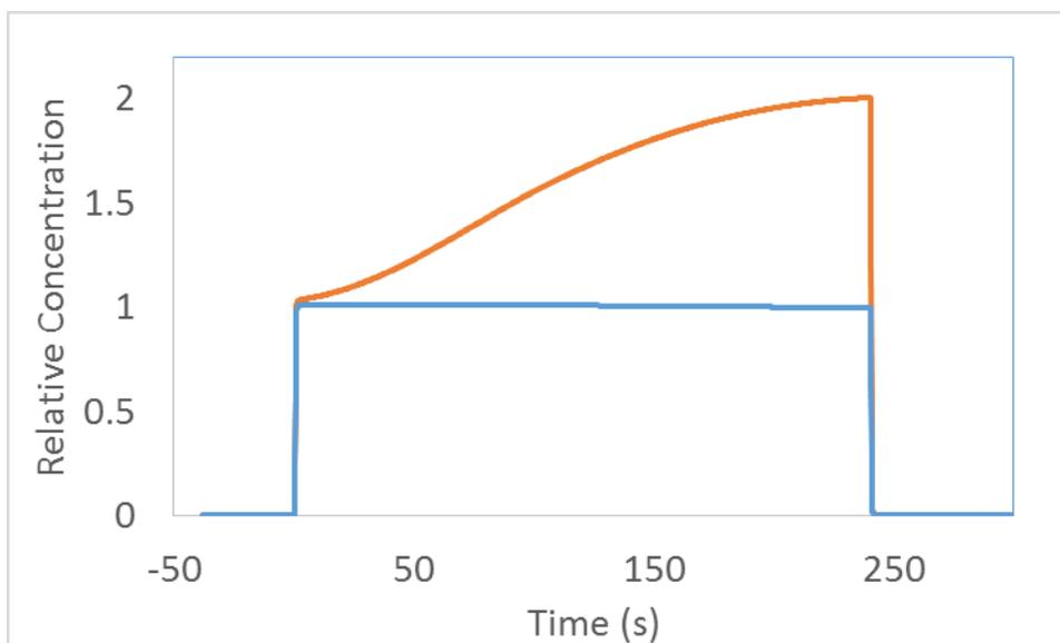
Figure 2A: Shows two NeXtStep injections overlaid: a gradient of ANALYTE (orange curve) in the constant presence of CONTROL and a constant concentration of CONTROL (blue curve) which is the reference (blank) injection.
