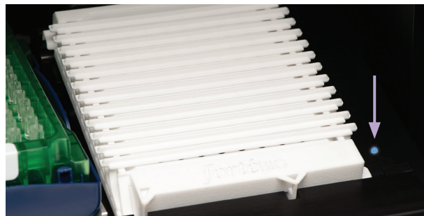
Figure 3: LED lights up when the evaporation cover is seated properly.
