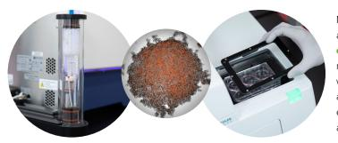
Microplates are placed in an environmental control cassette which introduces and maintains gas and humidity while reducing gas usage as compared to flooding the entire system. Cassettes can also be sterilized through UV.
