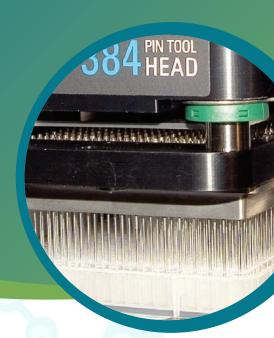
The FLIPR® High-Throughput Cellular Screening System includes a pin tool option for nanoliter liquid transfer. The pin tool pipettor is a complementary addition to the existing 96-, 384- and 1536-well pipetting options. When the system is configured with the pin tool, you get a cost-effective screening instrument capable of ultra high-throughput to accelerate your kinetic cell based assays.
