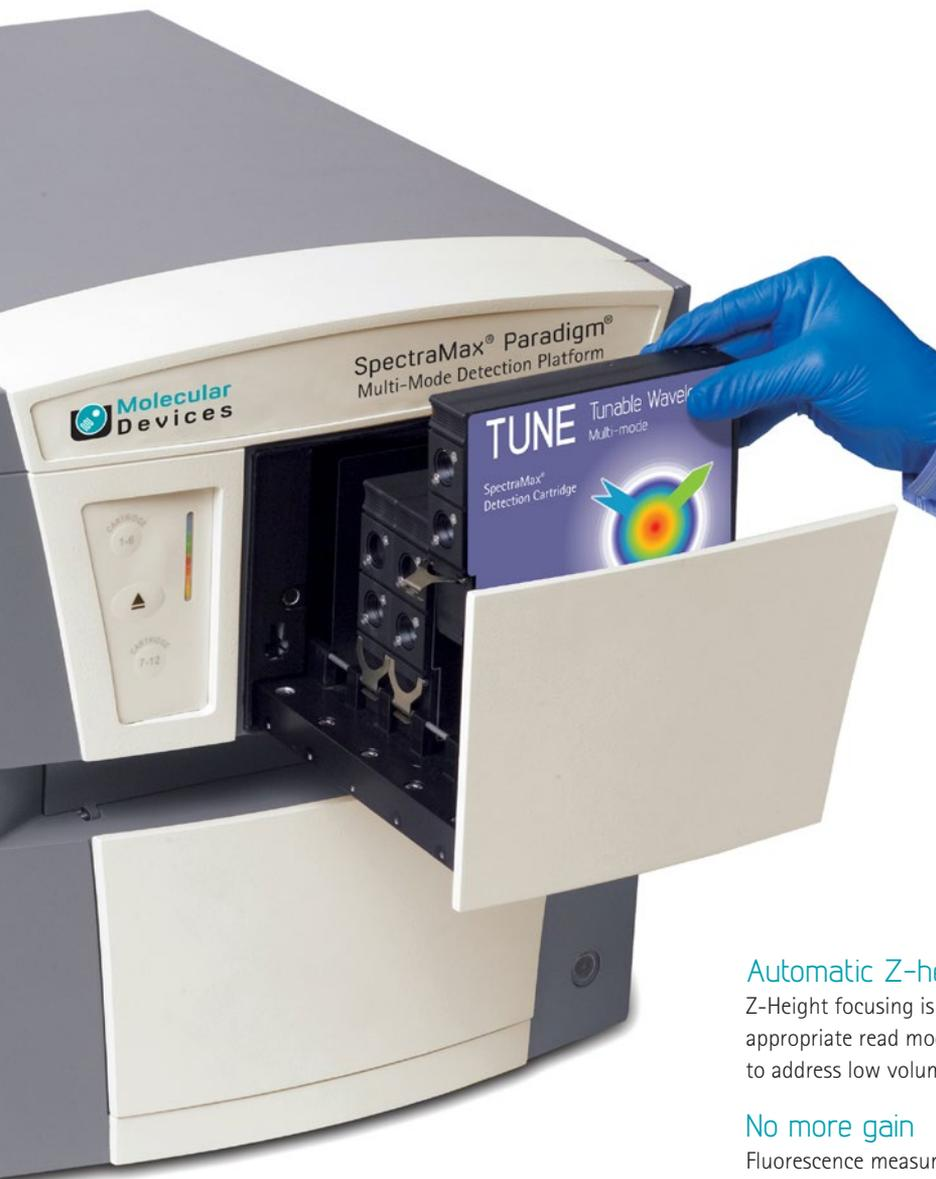
Every SpectraMax® Paradigm® Detection Cartridge starts with an application-optimized excitation energy source either in the form of a long-life, high-powered LED, xenon flash lamp, or high-powered laser. Concentrating the excitation light on the sample through label-specific optics, high levels of sensitivity and performance are reached. All this combined in the detection cartridge creates the ultimate no-compromise multi-mode detection platform.
