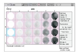
**Gemini XPS Reader scans.** Well scans from the Gemini XPS Reader illustrating serial dilution of CHO cells using the Live Cell assay from Molecular Probes Live/Dead (Calcein AM /Ethidium Homodimer-1) assay kit. A Costar 24-well tissue culture plate with col1 = blanks and doubling cell concentration left to right starting at Col. 2 with 1000 cells.
