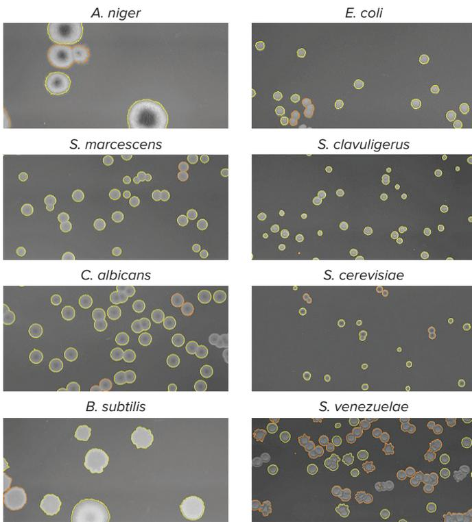
**Figure 2. Morphologically distinct colonies are identified by QPix colony detection algorithms based on user-defined parameters: compactness, axis ratio, size, and proximity.** Colonies surrounded by yellow border are selected for picking based on the user criteria, while colonies bordered with red fail to meet user-defined criteria and are excluded from picking.
