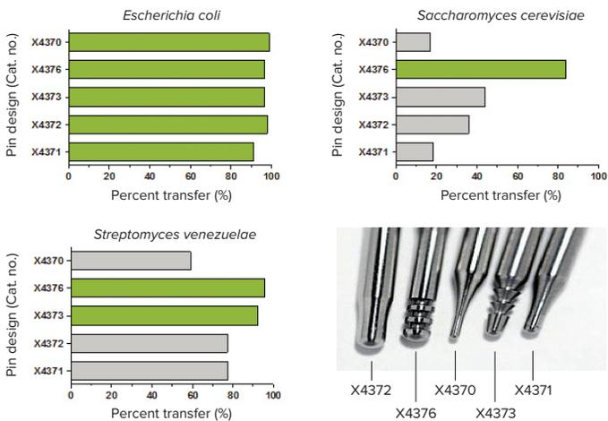
**Figure 1. Colony transfer efficiencies can vary widely according to the pairings between microorganisms and colony-picking pins.** A representative dataset is shown for *Escherichia coli*, *Saccharomyces cerevisiae*, and *Streptomyces venezuelae*.
