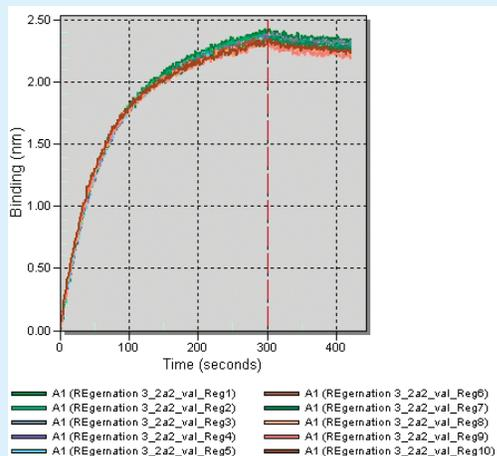
FIGURE 2A: Real-time binding chart of the development of regeneration conditions for Protein A-coated Amine Reactive biosensors binding to human IgG. Note no significant loss in binding capacity over 9 regenerations.
