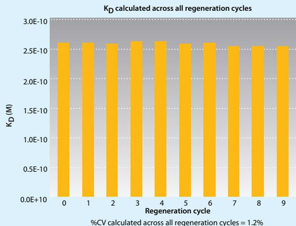
FIGURE 2B:  $K_D$  values calculated for each set of binding curves in Figure 2A using the Octet software. The reported CV is the coefficient of variance of the  $K_D$  from each set of binding curves across all regeneration cycles.
