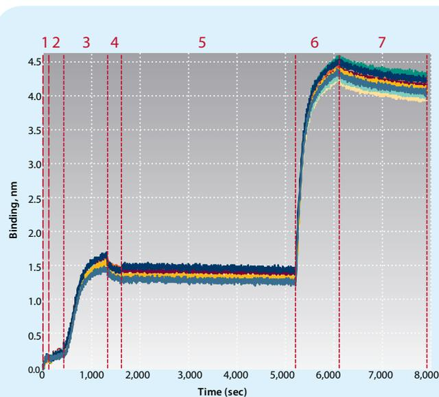
**FIGURE 1:** Immobilization of Protein A and binding of IgG to eight Amine Reactive biosensors in parallel on the Octet RED. The real time binding data shows all seven events during the experiment. 1 = baseline, 2 = activation with EDC/NHS, 3 = immobilization of Protein A, 4 = quench with 1M ethanolamine, 5 = baseline, 6 = association of human IgG, 7 = dissociation of human IgG.
