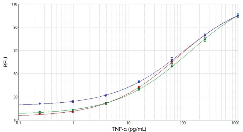
**Figure 3. TNF- $\alpha$  standard curves.** The 4-parameter curve fit in SoftMax Pro Software was used to plot data generated with SpectraMax iD3 (red), SpectraMax i3x (green), and SpectraMax M5 (blue) readers.
