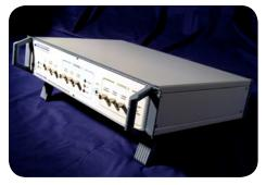
The Axon Axoclamp 900A Amplifier can be controlled manually or by software.
