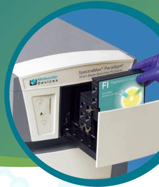
Fluorescence Intensity Detection Cartridges for SpectraMax® i3x and Paradigm® Multi-Mode Microplate Readers provide speed, sensitivity, and flexibility. The cartridge design provides uncompromising performance for both top and bottom reads. In addition, the standard dual-emission design enables simple, straightforward FRET (fluorescence resonance energy transfer) measurement.
