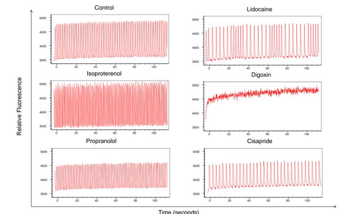
**Figure 7.** Calcium Flux assay using 3D cardiac spheroids treated with select compounds. Measurements done using FLIPR instrument. Phenotypic changes observed included: positive or negative chronotropic and inotropic effects with isoproterenol and propranolol, blocking of beating and Ca<sup>2+</sup> flux with digoxin, and beat irregularity with lidocaine. The vehicle control (0.3% DMSO) did not result in alterations of the beating pattern.
