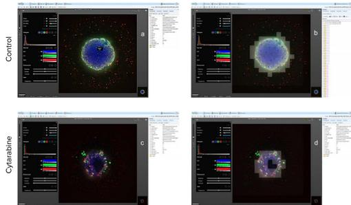
**Figure 5.** Example views of untreated (a,b) and treated (c,d) spheroid images. The untreated image (a) shows an overlay of manually scored locations separating centroid from non-centroid. The right hand images (b and d) show a mask overlay of blocks classified as spheroid. Only these blocks are used by a dose-response AI.
