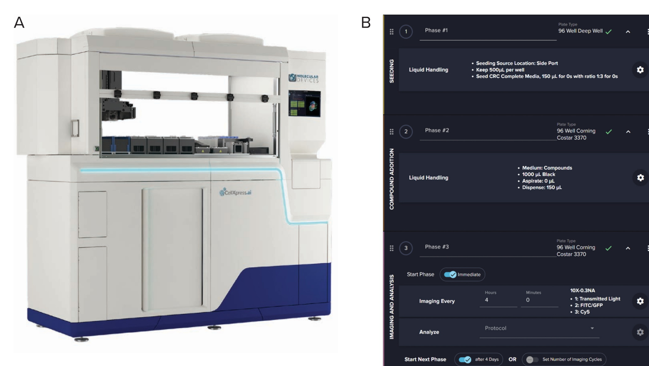
Figure 2. A. The CellXpress.ai Cell Culture System that integrates a liquid handler, an incubator with up to 154 plates, an imager with TL and up to 6 fluorescence channels and waste system; B. Three phases of Seeding from 96W deep well plate to 96W R 3 CE plate, Compound Addition from 96W compound plate to 96W R 3 CE plate and Imaging and Analysis workflow on the 96W R 3 CE plate.
