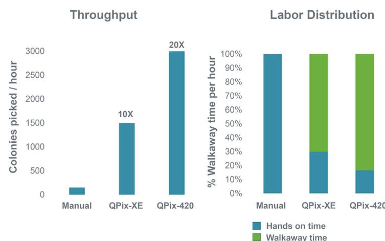
**Figure 2.** QPix XE has increased throughput and walkaway time compared to a manual screening and picking process. At half the speed of the QPix 420, the QPix XE was 10X more efficient at screening and picking colonies per hour with less hands-on time than a manual screening and picking process.
