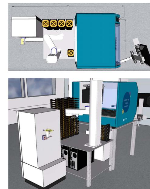
**Figure 5.** QPix XE function can be automated and integrated into a workcell. (Top panel) The 3D rendering shows a 3 ft x 7 ft automated workcell containing a QPix XE integrated with (top and bottom panel) a robotic arm to bring source and destination plates into and out of the QPix XE then to an automated incubator or ambient plate storage hotels.
