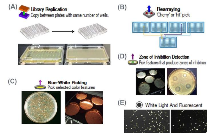
**Figure 4.** QPix XE applications. The QPix XE is capable of screening microbial colonies in many modalities such as (A) library replications, (B) Hit Picking, (C) Blue-White picking, (D) Zone of inhibition detection, and (E) Fluorescent detection. Other applications not listed can be easily licensed and added to software upon request.
