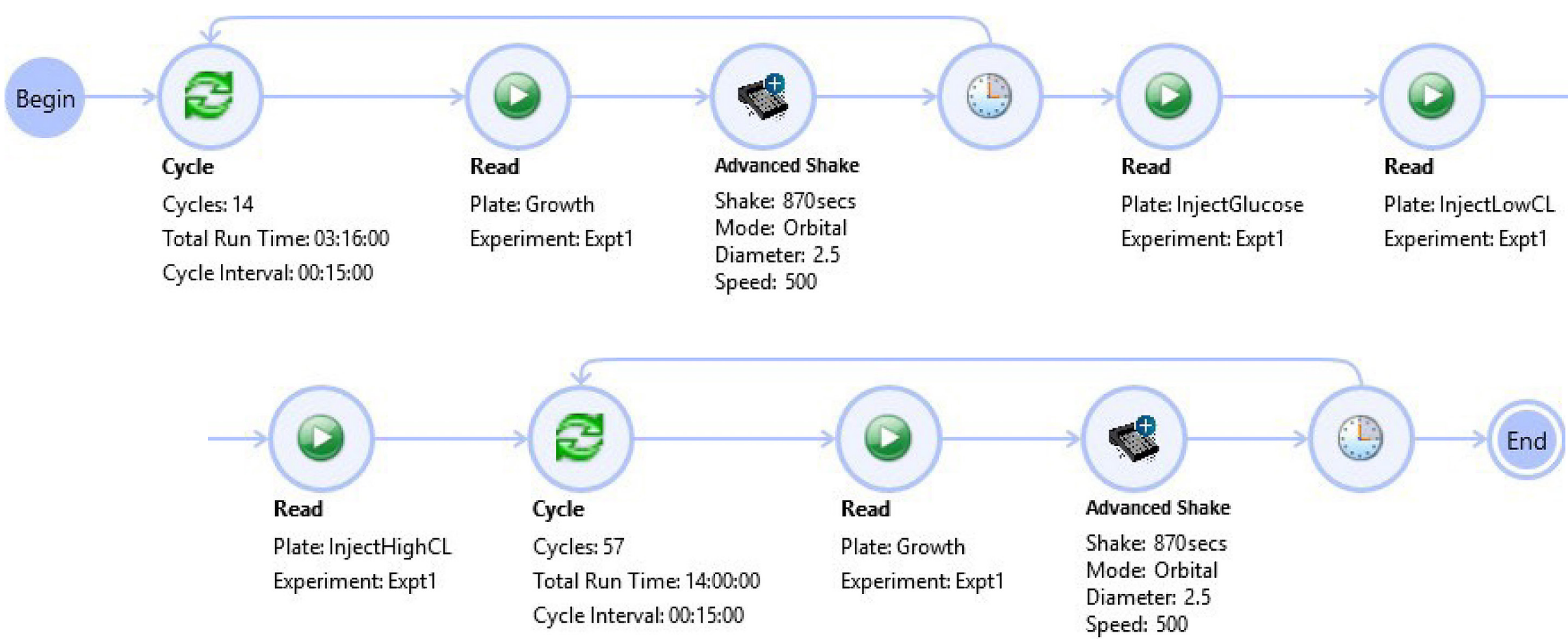
Figure 4. Workflow Editor in SoftMax Pro software was used to set up a three-part workflow: (1) 14 cycles of OD 600 reads followed by Advanced Shaking configured to match settings of a typical bacterial shaker (orbital mode, diameter 2.5 mm and speed 500 rpm); (2) injections of glucose or chloramphenicol into specified wells; (3) continuation of OD 600 reads with shaking. Total time: 14 hours.
