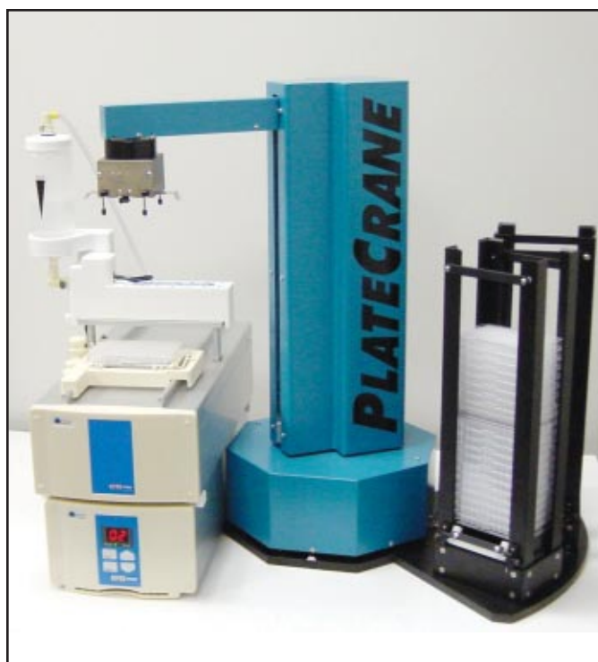
PlateCrane integrated with AQUAmax dispenser.
